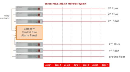
The flexible configuration options of the AP Sensing Linear Heat Series instruments allowed operators to quickly and easily define 7 independent alarm sections in line with the fire doors installed on each level of the parking garage
