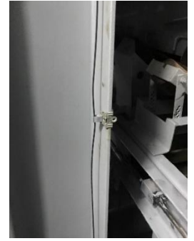
EM-SM beam clip can be used to fix the sensor cable on the conveyor belt
