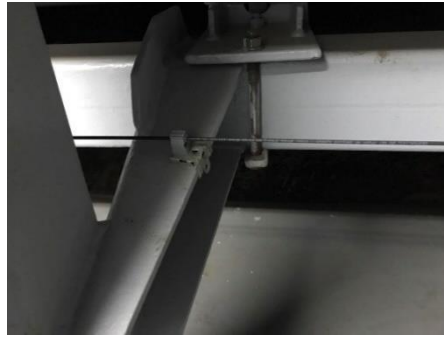
EM-SM beam clip can be used to fix sensor cable onto conveyor
