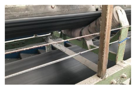
Cable installation (black), attached to the tension wire
