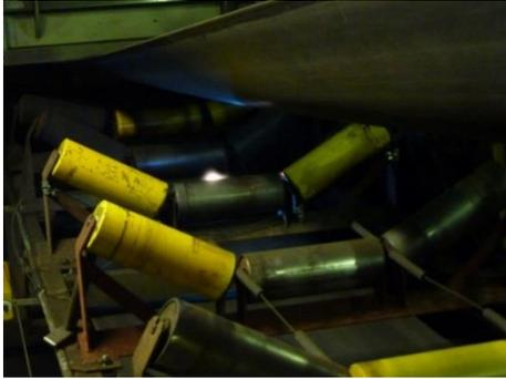
Figure 3: Sensor cable installation for detecting hot rollers
