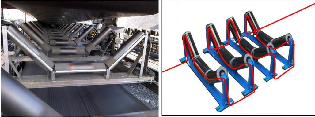
Figure 5: Mounting frame on an idler station and cable setup
