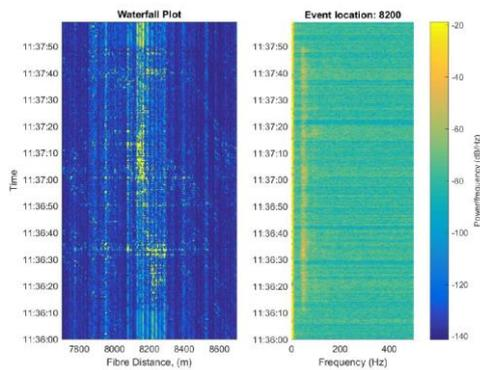
Figure 6: Acoustic response recorded by a distributed acoustic sensing system
