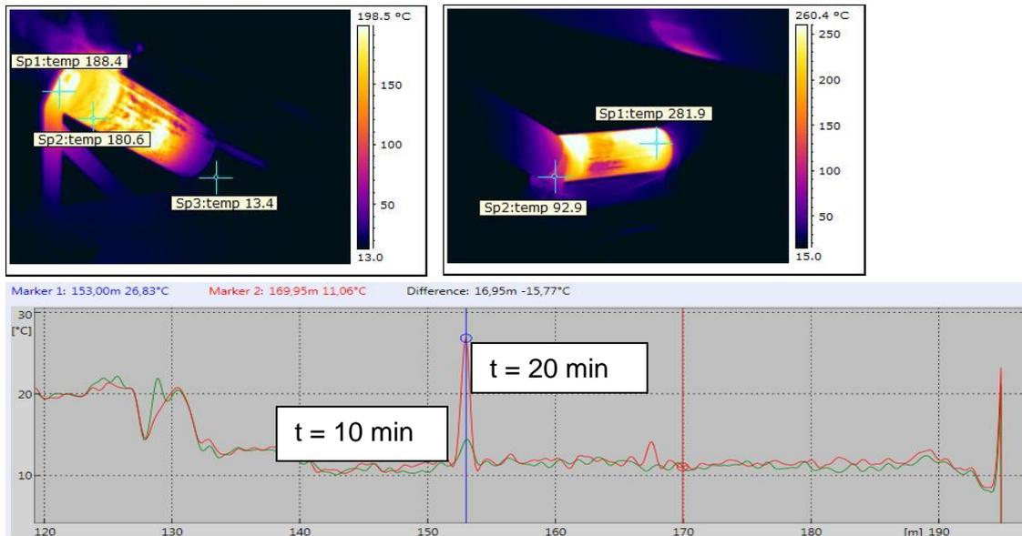
Figure 4: Temperature and DTS response of hot rollers
