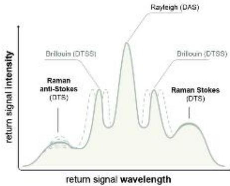
Figure 1: Optical spectrum of backscattered lines used by distributed sensing technologies
