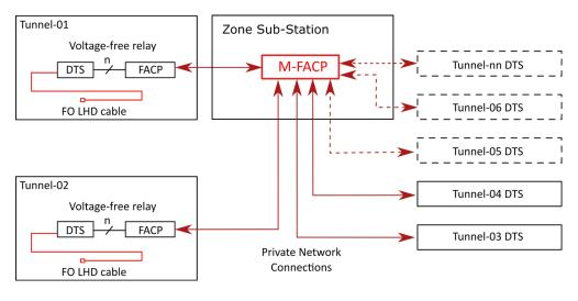
Each cable tunnel has been divided into individual fire detection zones, enabling the LHD to report the accurate location of a fire event to the FACP in real time. The systems were configured appropriately to ensure compliance to UL 521 and FM 3210 regulations.
