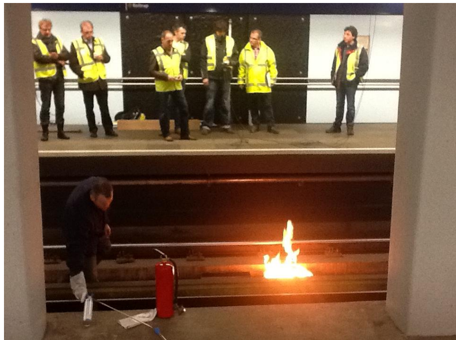
Heat detection test in the Rotterdam Metro
