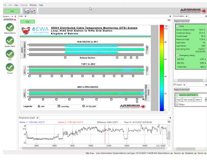
easy-to-use graphical user interface (GUI). Temperature graphs and hotspot tables are readily available, and circuit layouts are mapped and color-coded to show the measured cable temperatures and indicate any instantaneous changes. Sections of the cable route can be individually defined for flexible alarm levels and types, while points of interest (cable joints, horizontal drillings, manholes) can be analyzed with
