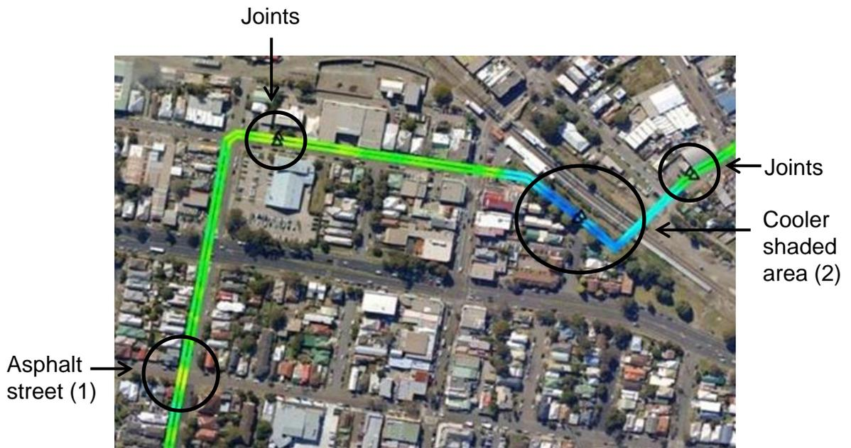
Gain insight along the entire installation by mapping GPS data together with the SmartVision asset viewer software. As shown above, even slight temperature changes can easily be seen when, for example, the sensor cable runs below a warm asphalt street (1) or it runs below a row of trees (2).
