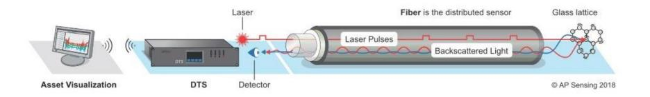
The Distributed Acoustic Sensing (DAS) is based on the **Coherent Rayleigh effect**, which is stimulated by minute strain changes in the fiber as a consequence of an **acoustic or vibration activity**. The returned signals are analyzed and presented in the form **of frequency and amplitude of disturbance**.
