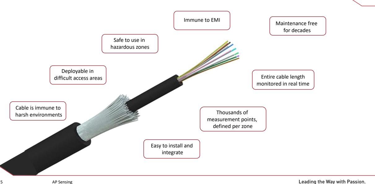
The Distributed Temperature Sensing (DTS) utilizes the **Raman effect** to measure the temperature. An optical **laser pulse** sent through the fiber results in some scattered light reflecting back to the transmitting end, where it is analyzed. The intensity of the Raman scattering is a measure of the **temperature** along the fiber.
