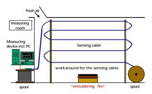
Fig. 5 longditudinal section through the breadboard construction including measuring system
