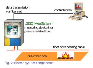
As a cost effective alternative to the shown seperate sections of transmission, separate fibers from the temperature sensing cable can be used for data communication.
