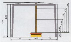
Fig. 4 cross section of a small fire drift with sensor cable system
