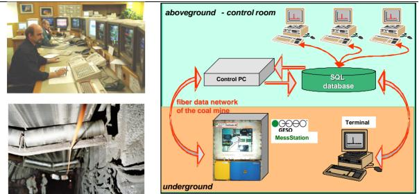
Fig. 9 The GESO Firefinder in the communication system of a mine
