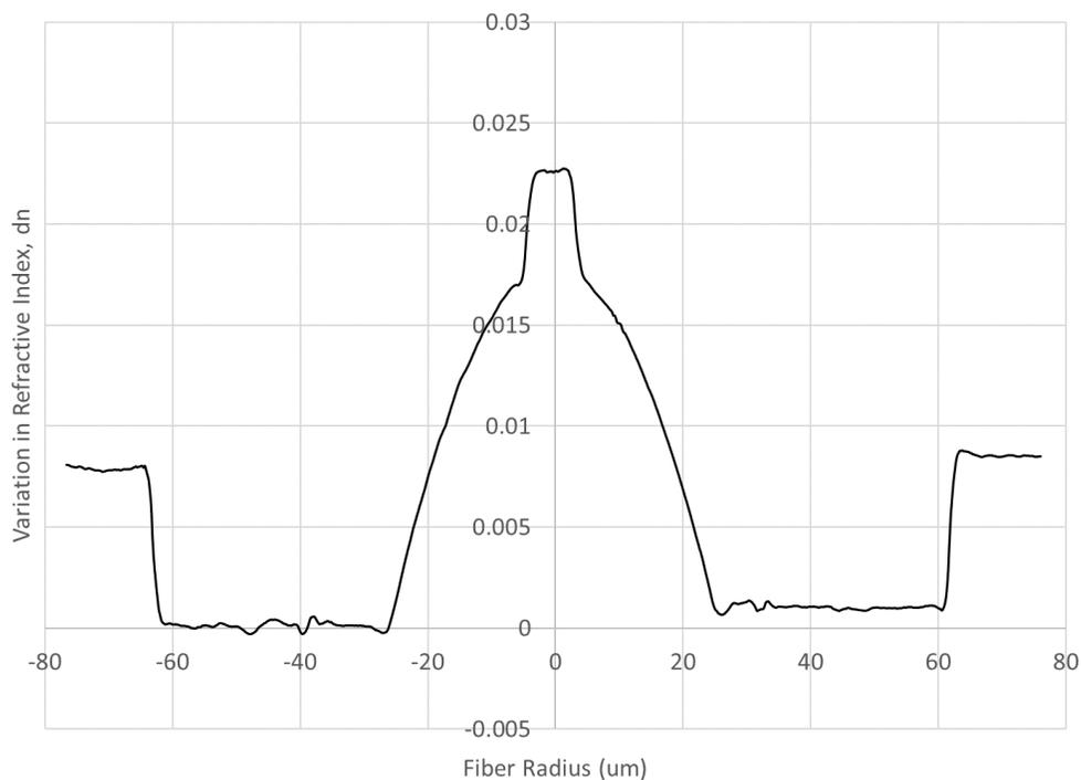
Figure 3. Refractive index of the DCGI(10.4/50/125) measured on an S14 refractometer.
