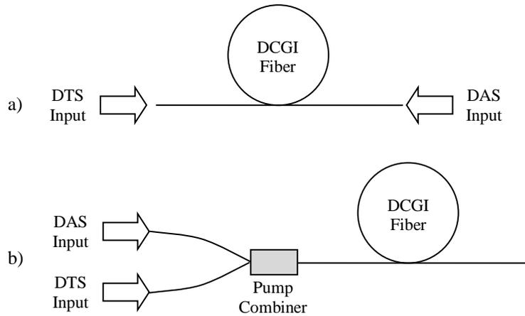
Figure 4. Experimental layouts for a) dual-ended measurements and b) single-ended measurements.
