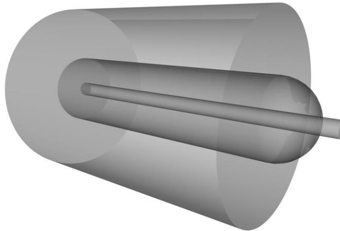
Figure 2. 3D CAD representation of the DCGI(10.4/50/125), showing the SM core, MM GRIN inner cladding and silica outer cladding. The coatings are not displayed.
