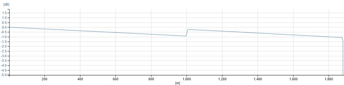
Figure 5. Attenuation plot at 1064nm from the AP Sensing N4586A DTS system showing 872m of the DCGI fiber after the 1,000m point.
