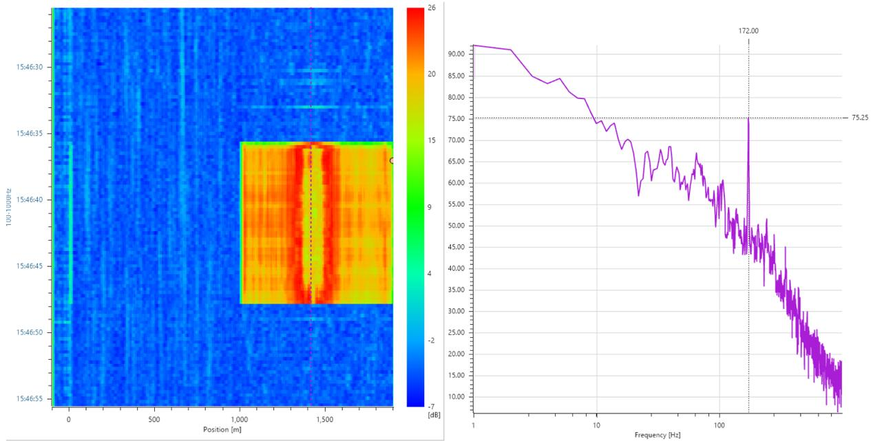
Figure 8. High frequency DAS test using a 172Hz vibration plate, showing the spatial and time response (left) and frequency response (right).
