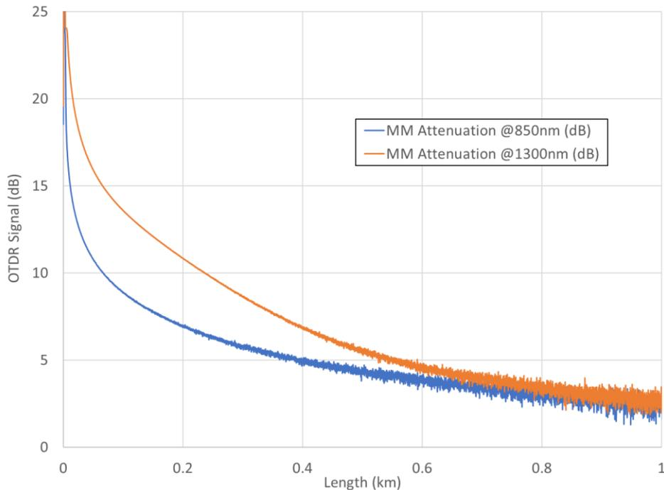
Figure 9. Distributed Rayleigh scattering of the MM core measured using an Exfo OTDR launched into the pump combiner.
