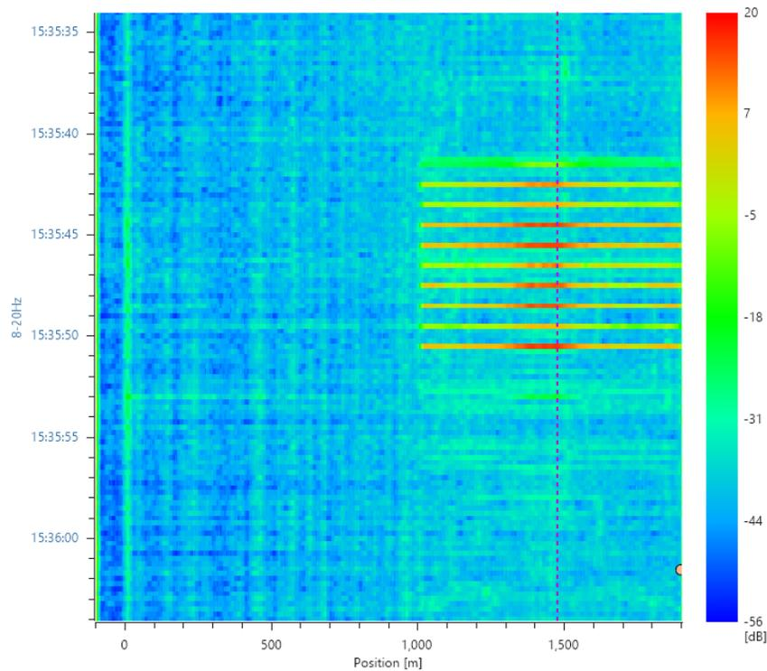
Figure 7. Waterfall plot of the generic MM fiber's (first 1,000m) and DCGI fiber's (>1,000m) DAS response within the frequency range of 8-20Hz over a duration of 30 seconds.
