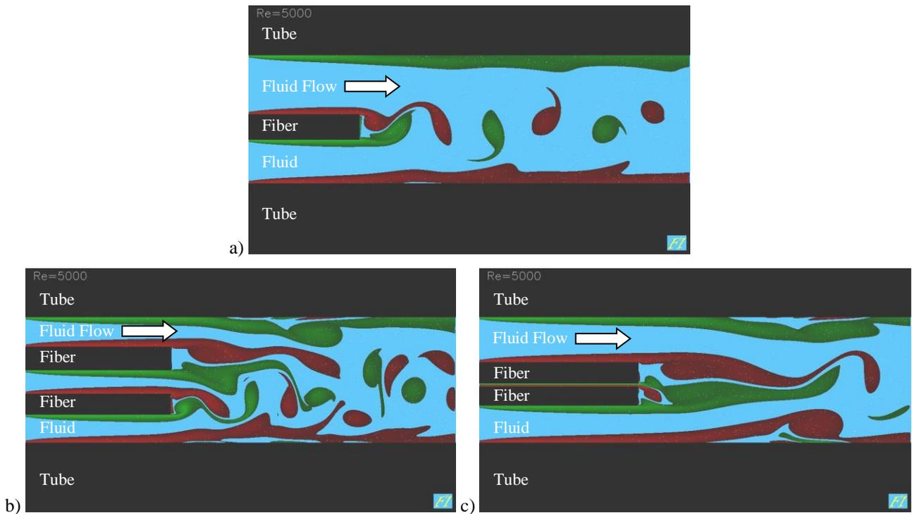
Figure 1. Illustrative representation of optical fiber pumping through a tube, based on fast solution of Navier-Stokes equations [6]. a) Single fiber, b) two fibers with a space between the two and c) two fibers in close proximity. Red colors indicate regions of high positive vorticity (rotating fluid particles) and green areas indicate large negative vorticity regions.
