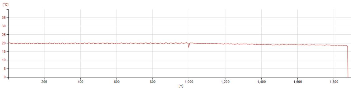
Figure 6. DTS plot at 1064nm from the AP Sensing N4586A DTS system showing 872m of the DCGI fiber after the 1,000m point.
