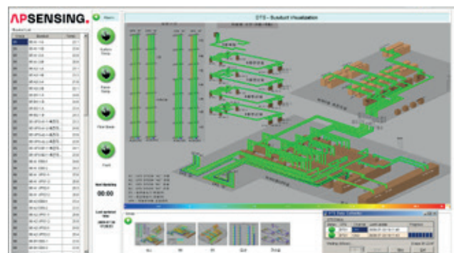
Visualization of bus duct temperatures
